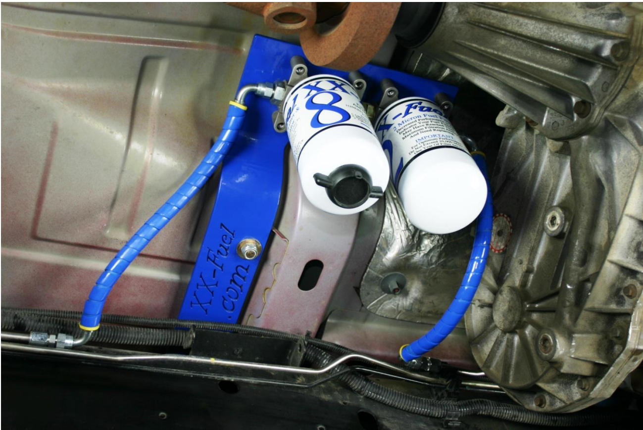
LongBed QuadCab or MegaCab Installation showing optional fuel line cut position
